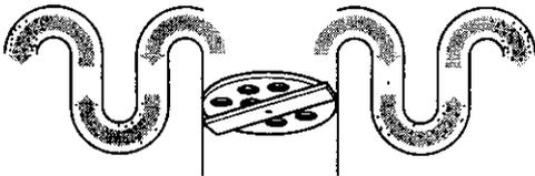
9. Fresh, hot water enters the dishwasher and sprays on the dishes. The rinse water is then pumped through the soil removal system and remaining soil is removed.
