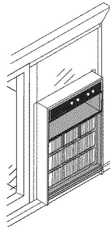
**14. Drill two 9/64-inch diameter pilot holes** in the top window jamb in line with the partially plugged holes in the panel frame. Secure the panel frame to the window jamb with two #8-32x3/4-inch self-threading screws. If additional holding is necessary, two screws may be used on the sides of the panel frame as well.
