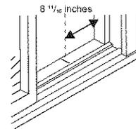
Apply track seal to the outside edge of the bottom window jamb.
