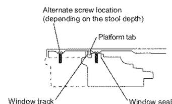
Center platform assembly on the line with platform tab pressed against window track
