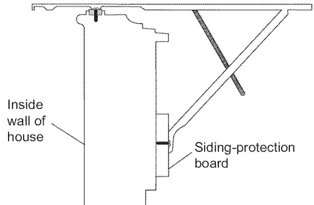
**6. Place platform assembly**, with platform tab against inside of window track, and attach it to window jamb. Use appropriate length screws (Items 9-11 in Preparing For Installation).
